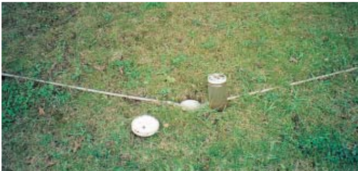
Figure 3. Tube-type lawn sampler (site 2).
